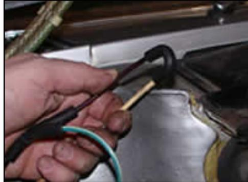
**NOTE: Spray the car's vacuum connector with a light coating of synthetic lubricant before inserting any of the vacuum lines. This will make it easier to remove the connections in the future.**
