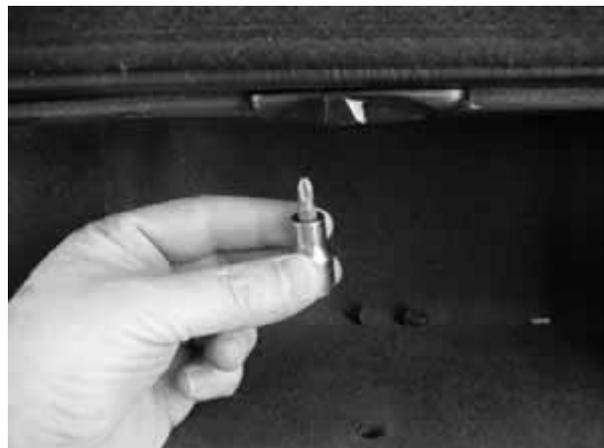
You can also remove the glove box door to gain additional space to maneuver. This is done by removing the Philips head screws attached to the hinges and the screws attached to the sides of the door. Be sure to keep track of all these pieces for reassembly!
