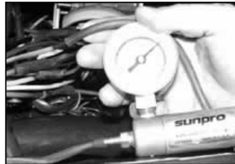
**NOTE: The Controller Box does not have the ability to turn off the Blower nor does it control the A/C Compressor Clutch. If the Blower or the A/C compressor are not operating normally then there's a vacuum leak. The GREEN vacuum circuit requires at least 6in Hg to turn on the blower. Call UnwiredTools if you have any questions about troubleshooting the vacuum system.**
