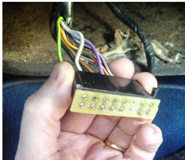
Jumper block shown installed on the Servo Amplifier connector. **Be sure the match the color abbreviations to the wire colors so that the jumper block is not installed backwards!**
