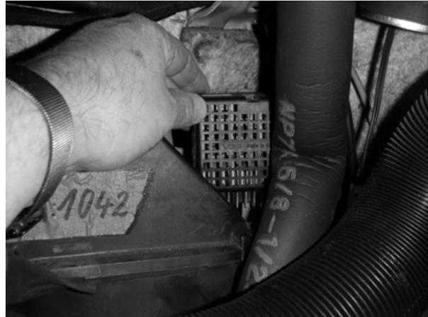
With the Servo Amplifier removed, the next task is to install jumpers across terminals of the Amplifier connector. This connection is made in one easy step using the jumper block PCB, which is included in the kit. When this jumper block is installed the effect is as follows:
