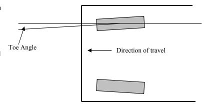
This stable feel comes at a cost. A positive toe setting means that the tires are pointed very slightly inward. This inward angle means that both tires are slightly skidding sideways to overcome the positive toe setting. This effect can be very significant.
