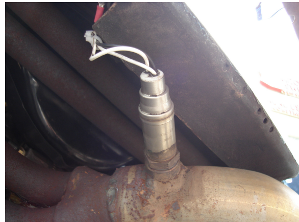
Bosch 13913 installed in bung welded to header
