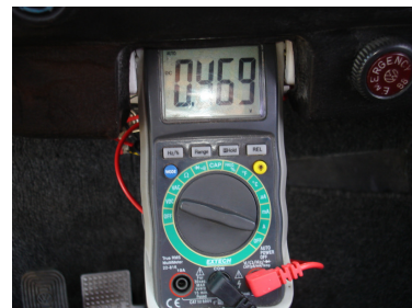
Volt meter reading oxygen sensor in volts
