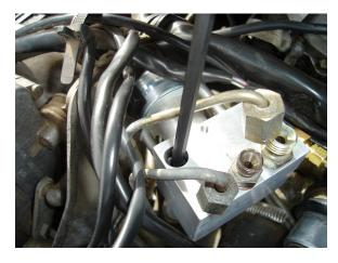
Now tighten the fuel fittings on the top of the valve assembly then tighten the fuel lines. Note: The fuel lines must be properly torqued, not over-torqued, to prevent leaks. Use a backing wrench as shown to properly tighten the fuel line nut onto the fitting. The body of the UTCIS™ is aluminum, DON'T STRIP THE THREADS!!
