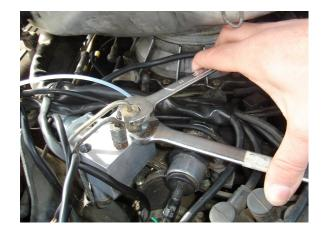
The UTCIS-PT<sup>™</sup> has a vacuum connection which can now be connected to any source of intake manifold vacuum.
