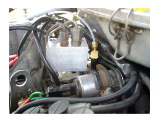
Plug in the red bullet connectors to connect the RPM sensor to the controller. Pass a sparkplug wire through the center. It does not matter which sparkplug wire is used.
