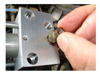
The body of the UTCIS™ regulator can now be mounted in the same location as the OEM part. The aluminum spacers in the hardware kit are used to position the UTCIS™ at the same height as the OEM regulator. Tighten the M6 x 65 mm screws as shown. These screws thread into the same mounting points as the OEM Warm-up Regulator.
