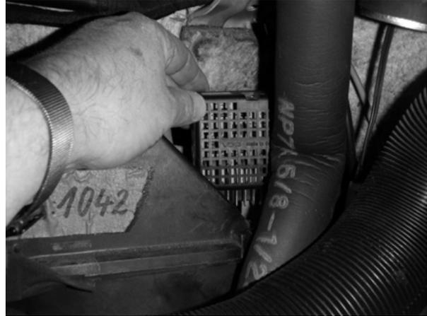
With the Servo Amplifier removed, our next task is to install jumpers across terminals of the Amplifier connector. The connector is keyed so you can determine which side is position 1. There are a total of eight positions on the connector. Obtain the 3 jumpers found in the Electrical Hardware Kit. Install jumpers across positions 1 to 2, 3 to 5, and 7 to 8 as shown below.
