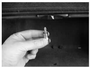
The glove box light can be removed by inserting a thin screwdriver edge at the front then gently prying down and toward the rear. When the light is removed from its hole the glove-box liner may be removed.
